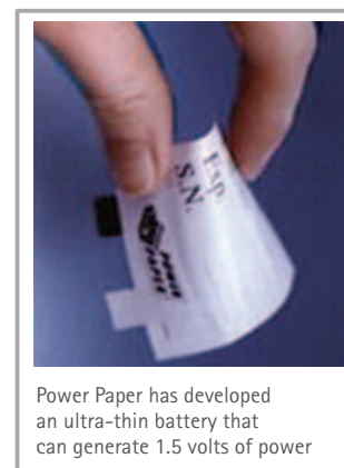
Figure 25. Ultra Thin Paper Battery Source: Power Paper
